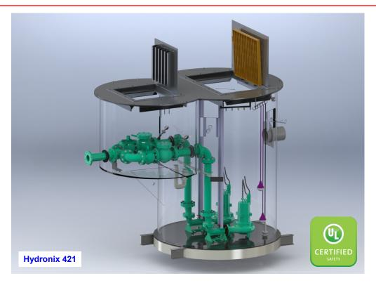
The Hydronix 421 is an engineered, fiberglass wet well and valve vault that is molded as an integrated unit. A durable gel coat protects the exterior while a smooth, white gel coat on the interior allows for high visibility and easy wash down. Wall thickness is engineered for each application and provides a minimum life expectancy of 50 years.
