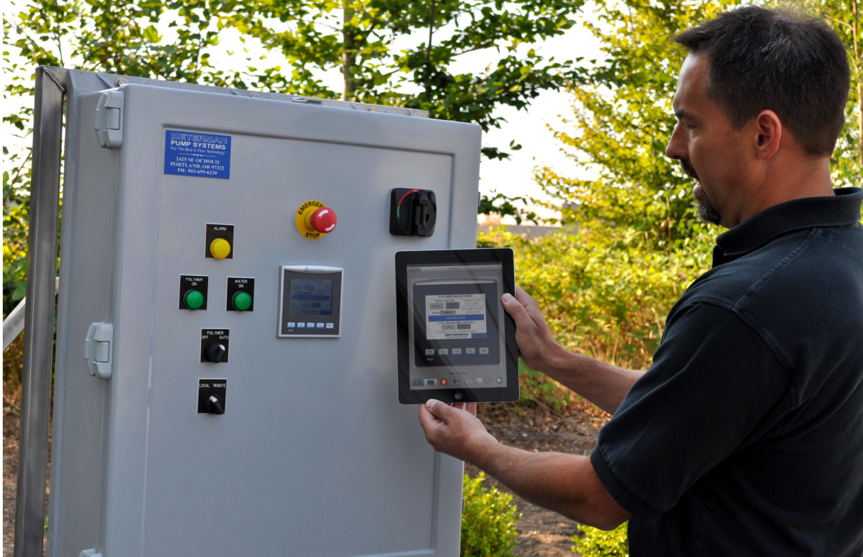
Apple iPad connected to a Unitronics V350 PLC via iRover
